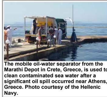
The mobile oil-water separator from the Marathi Depot in Crete, Greece, is used to clean contaminated sea water after a significant oil spill occurred near Athens, Greece. Photo courtesy of the Hellenic Navy.
